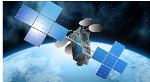
**Figure 1.** A commercial HTS spacecraft employing multiple Stellant Systems Q-band LCTWTAs.
