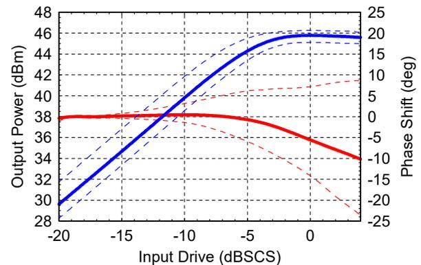
**Figure 4.** 2000HDA 35-W Q-band LCTWTA measured output power and phase vs. drive for the flight set.
