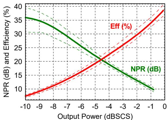
**Figure 3.** 2000HDA 35-W Q-band LCTWTA measured NPR and efficiency versus output power for flight set.
