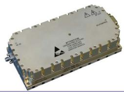
Comtech PST has announced the release of a solid state Class "AB" linear amplifier which operates over the full 2500-6000 MHz frequency band and delivers a minimum of 50 watts. The amplifier uses the latest Gallium Nitride (GaN) technology and is housed in a relatively small package measuring only 7.5" x 3.0" x 1.5" (excluding connectors).
