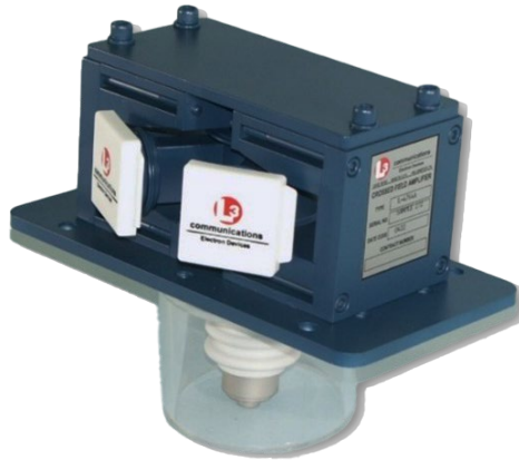
Fig. 4. L4764 X-band radar crossed-field amplifier (0.5 MW, 9.5 -10 GHz, 0.001 duty). Dimensions are approximately 8.5 x 12 x 5.75 in (height, length, width). Nominal operating voltage is 35 kV.
