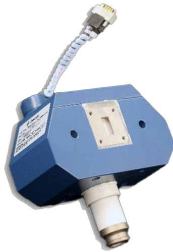
Fig.3. L4649 High power Ku-band frequency agile magnetron. Nominal operating parameters: 14 kV, 10A (pulsed), 85 kW peak power, 225 MHz frequency tuning range (min), max duty 0.0006.
