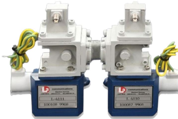
Fig. 2. L4110/L4111 Ku-band injection locked magnetron set (each magnetron is 4 x 2 x 1 in, not including circulator). The separation distance between magnetrons is 1 in. RF input and output ports are SMA, with an isodaptor at the input and a W/G to coax transition at the output.
